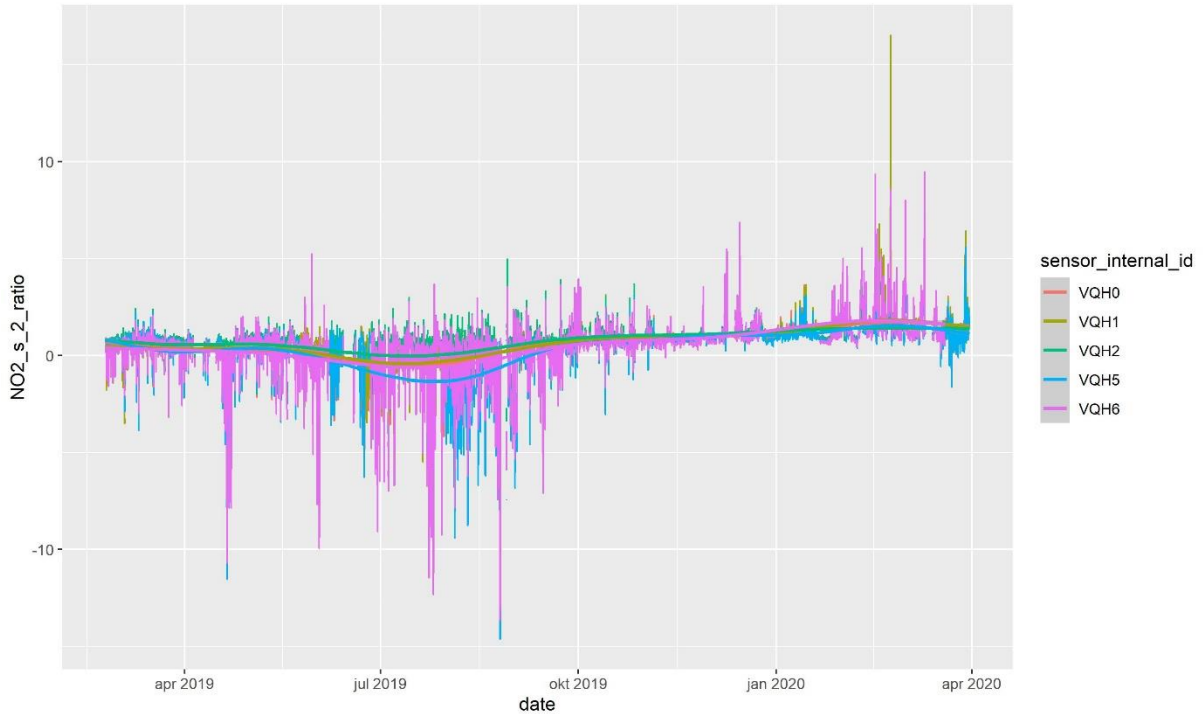
Figure 19: Alphasense B43F NO 2 sensor: Time plot ratio sensor hourly values versus reference values (µg/m 3 )
