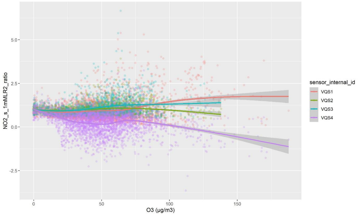
Figure 126: Envea Cairclip \text{NO}_2 sensor: Scatter plot ratio sensor hourly values calibrated with multiple linear regression versus reference values in relation to ozone ( \mu\text{g}/\text{m}^3 )
