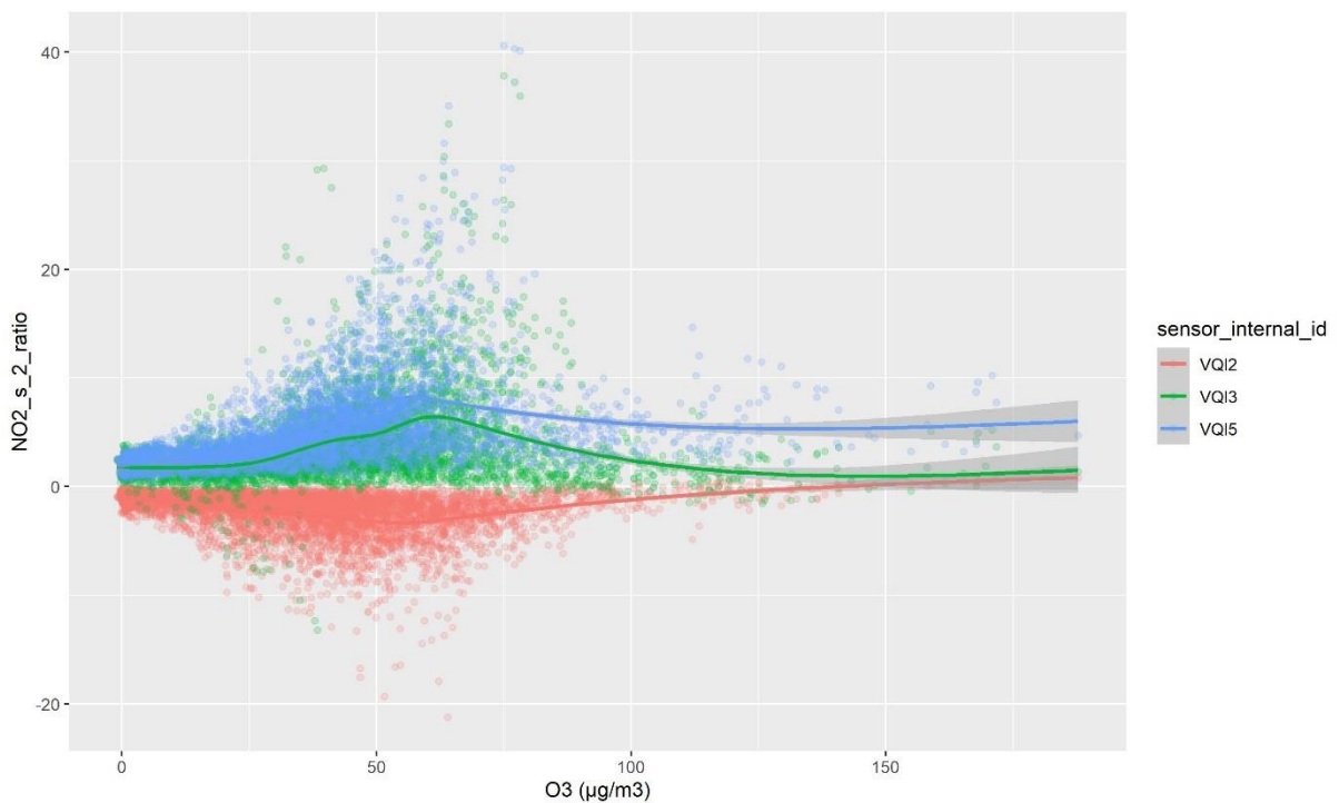
Figure 53: Citytech 3E50 NO 2 sensor: Scatter plot ratio sensor hourly values versus reference values in relation to O 3 (µg/m 3 )
